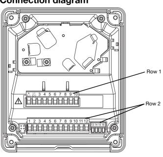
The connection diagram in the data sheet provides preliminary information about the connection options. For the electrical connection, only use the installation instructions or the operating manual. The knowledge and the correct technical execution of the safety information/instructions contained in these documents are mandatory for mounting, electrical connection, startup, and for safety during operation.
