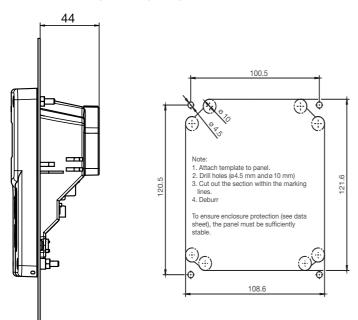
Note: The drilling template is shown actual size in operating manual B 202566.0.
